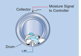
A low voltage current is passed through the laundry by specially insulated lifters. The moisture is measured 400 times per second.
